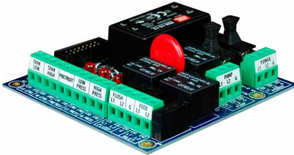
Figure 4. Controller Detail: Terminal Board, TB-6 (See Fig. 1 for schematic)
